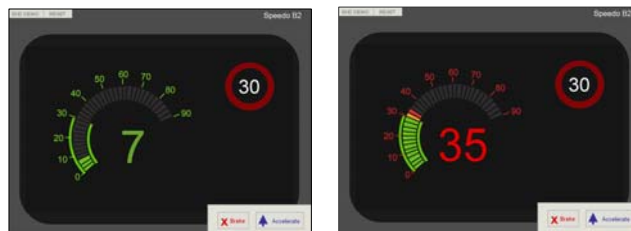
Example speedometer displays showing speed limit and non-compliance information
