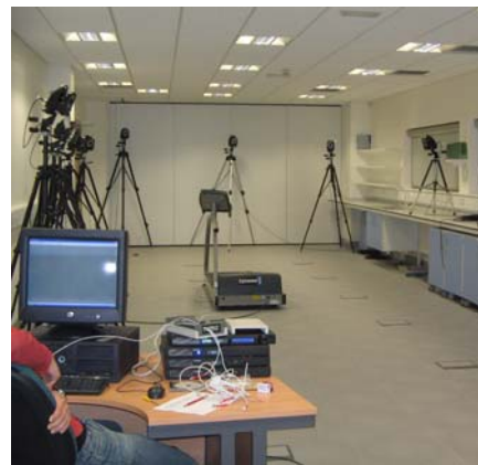
The Vicon system measured 3D position of reflective markers placed on the body
