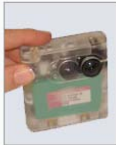
The v2.3 SenseCam shown close up and as typically worn by a user. The model pictured here has a clear plastic case that reveals some of the internal components.
