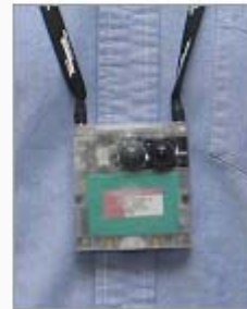
The v2.3 SenseCam shown close up and as typically worn by a user. The model pictured here has a clear plastic case that reveals some of the internal components.
